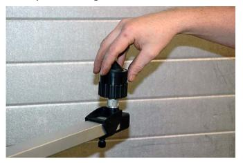
3. Lock the height measuring rod to the arm.
