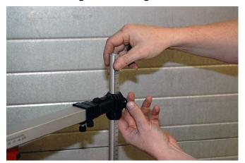
4. Snap in tip/cup to height measuring rod.
