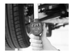
Before starting to measure it is important to secure the setting of the measuring arm. This is done by compressing the arm altogether and pushing the ON/0 button until the display goes off. With the measuring arm still compressed push the ON/0 button and the digital number 900 (900mm) will appear. The measuring tool will now measure according to this setting and always start measuring from 900 mm.
