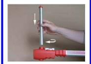
Collapse the telescoping measuring arm completely and press the "On/O" on the display panel. A digital number 900 (900mm) will appear in the display window representing the minimum collapsed length of the arm between centres.
