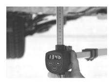
Repeat the same procedure on the other side of the vehicle's corresponding and selected symmetry (cross) measurement point (measuring line no 3).
