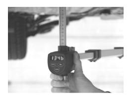
Before starting to measure it is important to check the setting of the measuring arm, see 4.3 LENGTH MEASURING.
