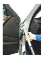
**Mount**Place the gap around the welded door hinge
